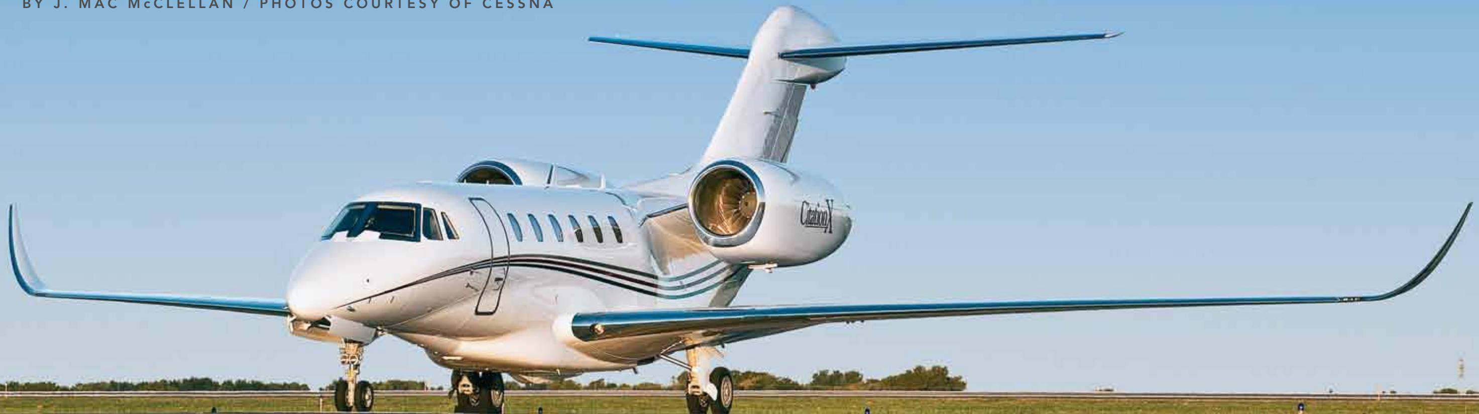
With its limit speed of Mach .92 the X can cruise up to about 528 knots true airspeed. A more typical fast jet cruise speed is around Mach .82, which equals about 470 knots. And lots of jets, particularly the extremely popular Boeing 737, cruise well under Mach .80, which is 459 knots. The Citation X does stand out.
